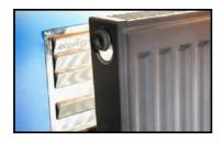
**Radiator reflector panels:** These are a low-cost energy efficiency option. Fixed behind your radiators, they reflect heat from the radiator back into the room, instead of letting the heat out through an external wall. They have most benefit when installed on un-insulated walls. Also make sure radiators are not obstructed by curtains or furniture.
